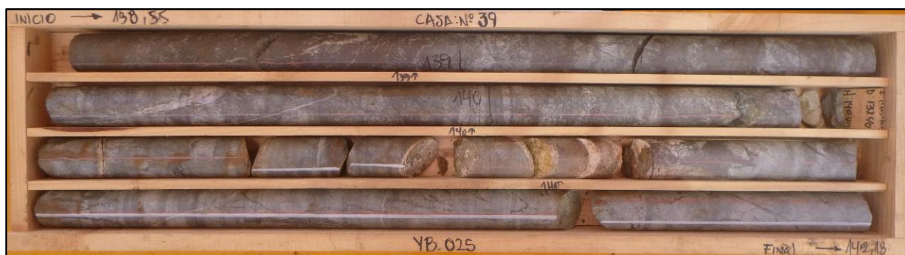
Figure 1 - Core tray 39 from diamond drill hole YB025 showing typical high grade magnetite mineralisation – interval 138.5m to 142.2m shown
