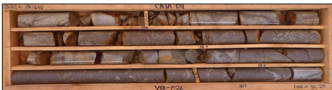
Figure 2 – Core tray 04 from diamond drill hole YB026 showing typical high grade magnetite mineralisation – interval 26.2m to 30.2m shown
