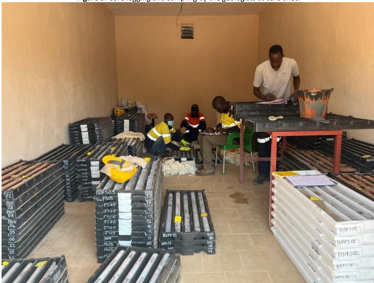
Figure 9: Core logging and sampling by the geologists at core shed.
