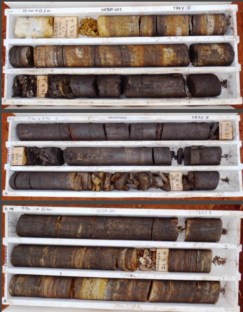
Diamond core hole OKDM002 17.5m to 19.9m. Massive manganese with minor manganiferous shale logged from 16.7m to 20.8mm
