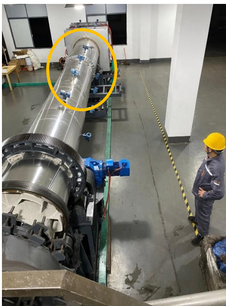
Image 2: Calcining Kiln with temperature gauges highlighted
