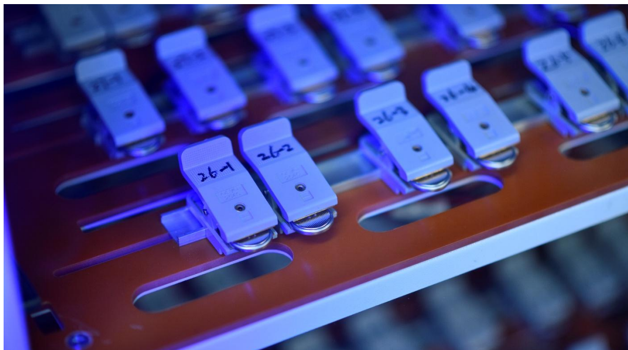
Figure 1. Cataloguing coin cells for electrochemical testing, manufactured using Firebird's LMR technology.
