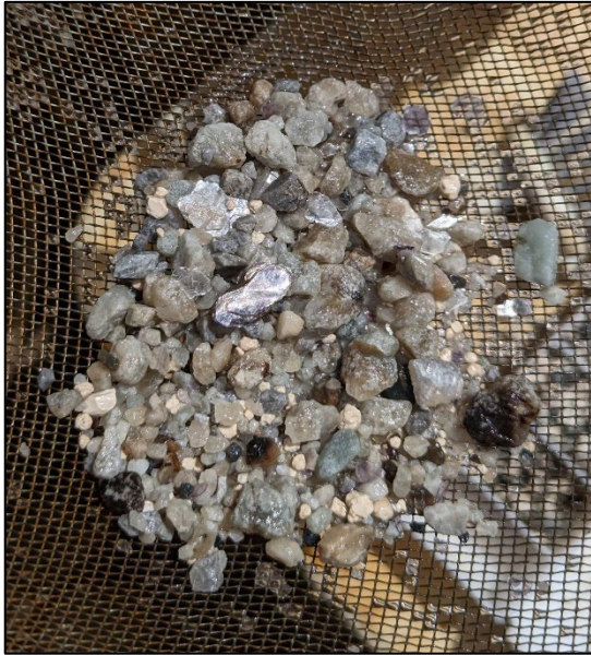
Figure 11: Lepidolite and cookeite bearing pegmatite in FGER0007 at 59m depth
