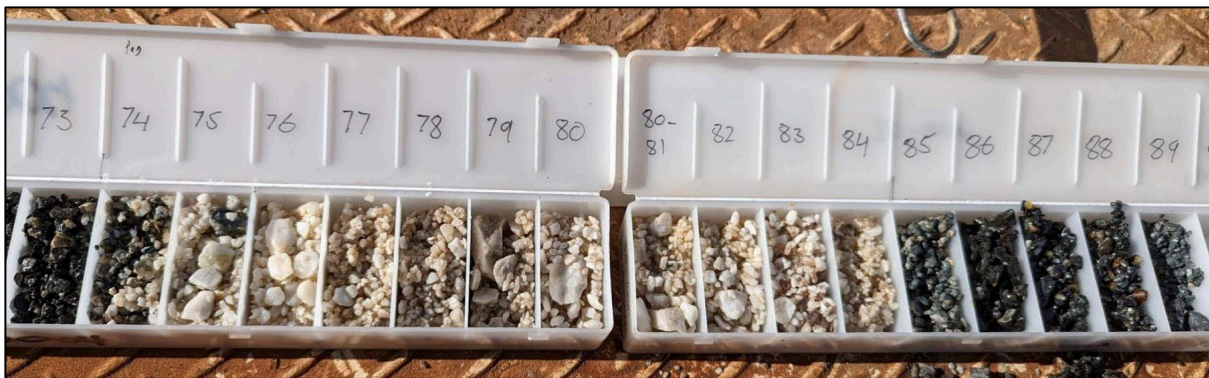
Figure 5: FGIR0004 chip trays showing 11m of pegmatite from 73m
