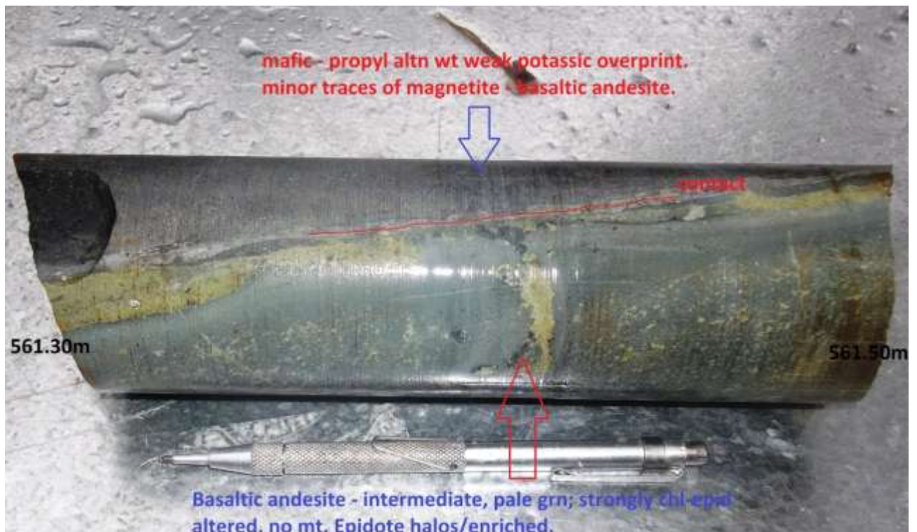
Photo 2: Contact zone, epidote rich basaltic andesite in contact with weak potassic overprinting zone.
