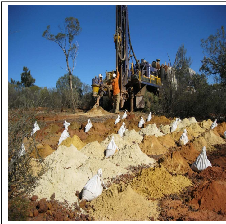
Figure 2: RAB drilling, September quarter 2010
