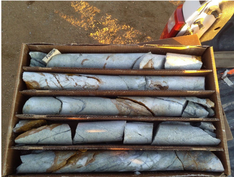
Core from GDD02 from 584 ft to 593 ft downhole. Stockwork and sheeted quartz-sulphide veins. Quartz-sericite-pyrite alteration.
