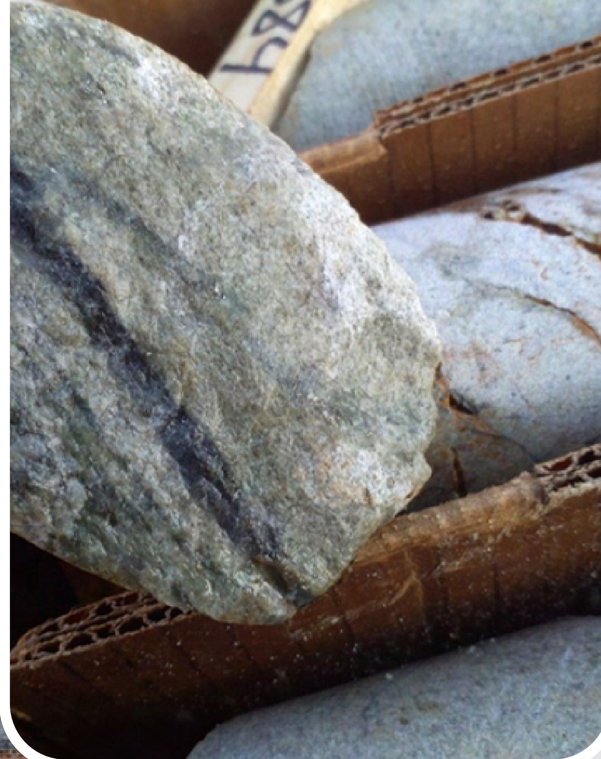
Left Image: Core from GDD02 from 178 m to 181m downhole which assays 40 g/t Gallium Stockwork and sheeted quartz-sulphide veins. Quartz-sericite-pyrite alteration
