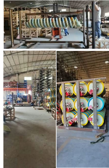
Spirals being assembled at factory and place in supporting skid for shipment to Dolphin
