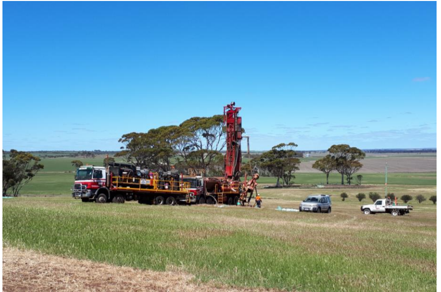
RC drilling over EM Anomaly 2 at Quicksilver
