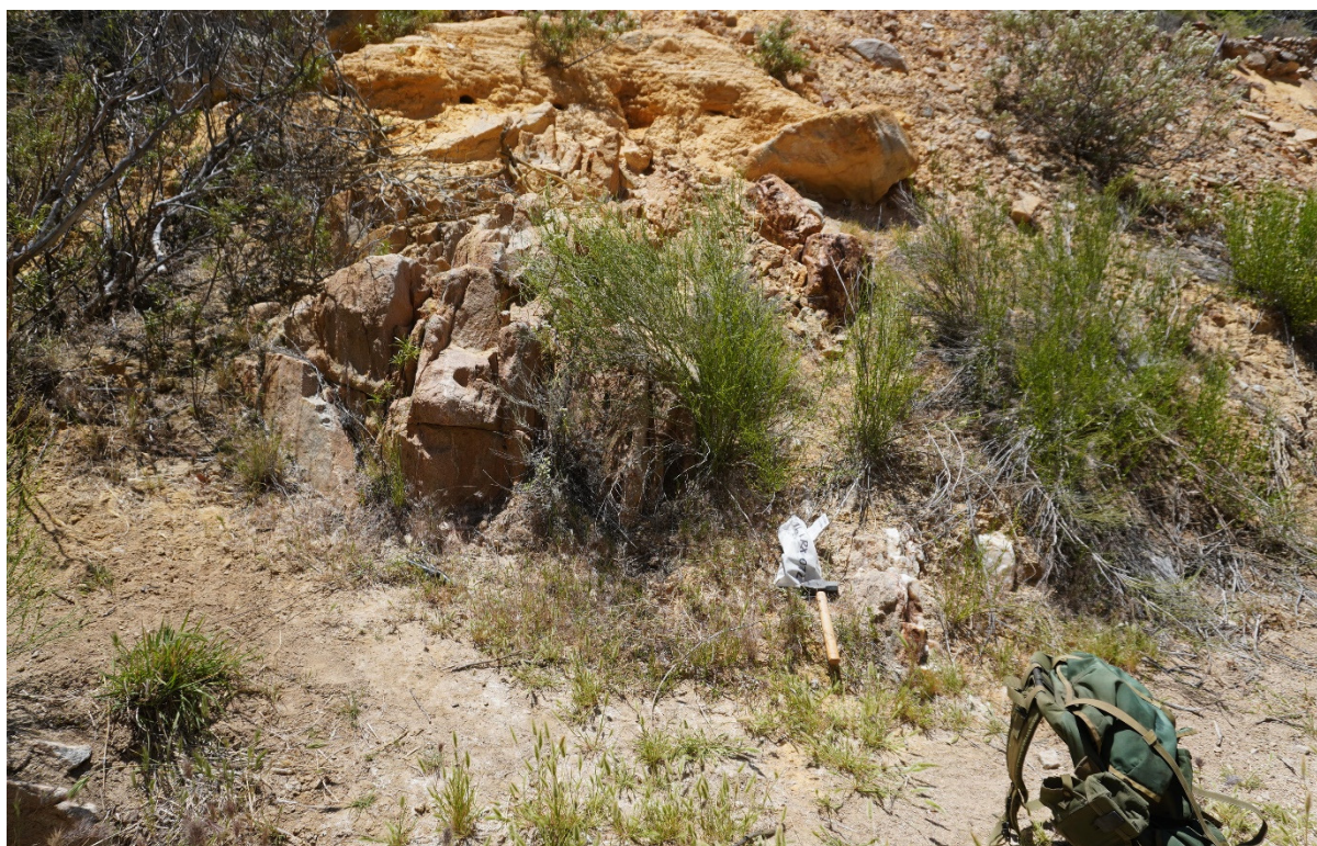
Figure 6: Sample 26 LRX 072 location showing intense hydrothermal alteration (sample assayed 8,300ppm Cu)
