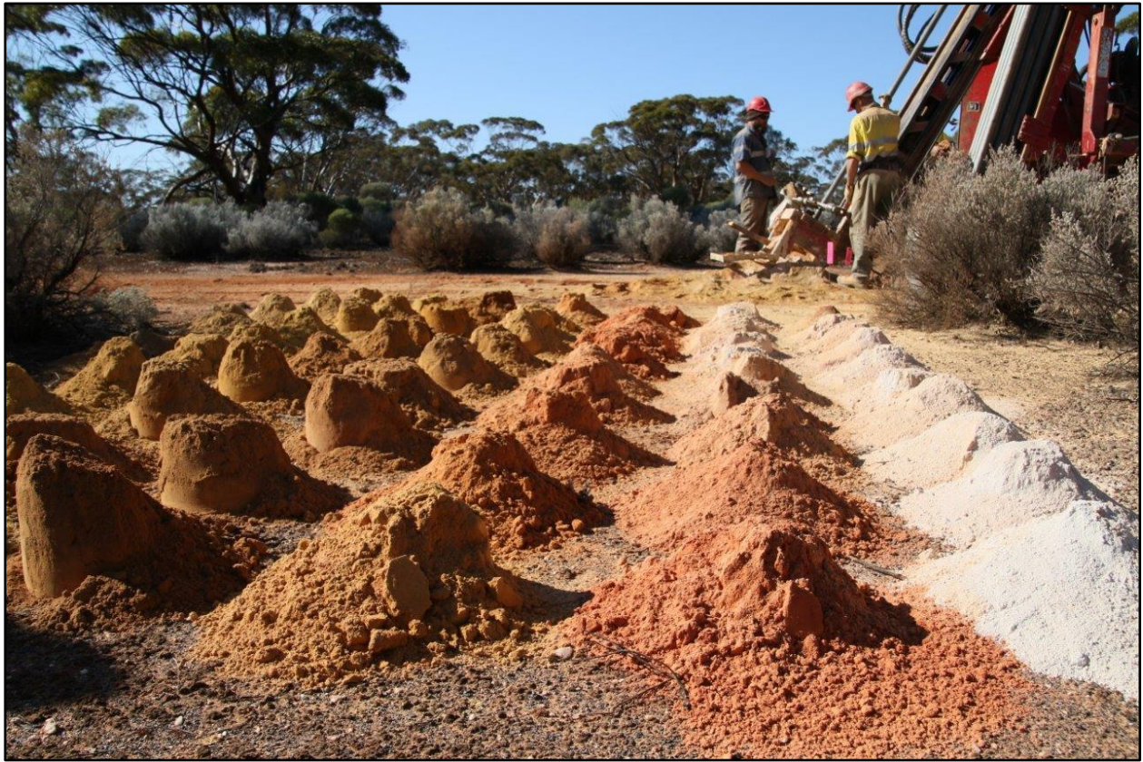
Figure 3: RAB Drilling at the Zuleika JV.
