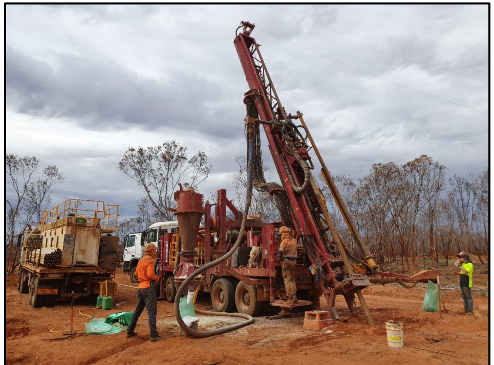
Figure 1 – RC Drilling Rig at Galileo's Lantern Prospect in the Fraser Range
