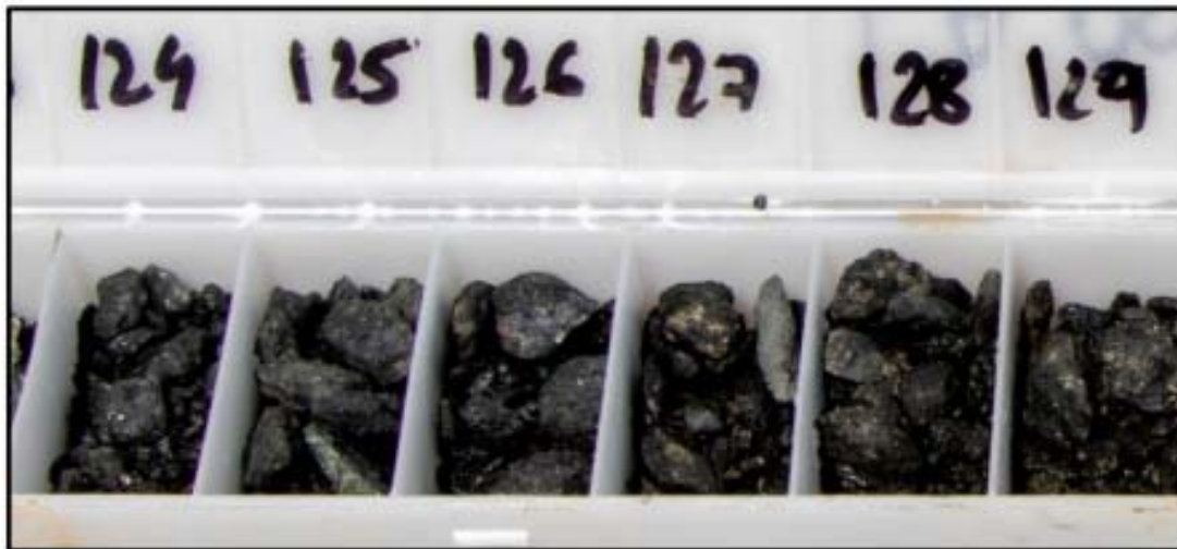
Figure 3: RC drill chips from LAARC003 showing sulphide rich mineralisation
