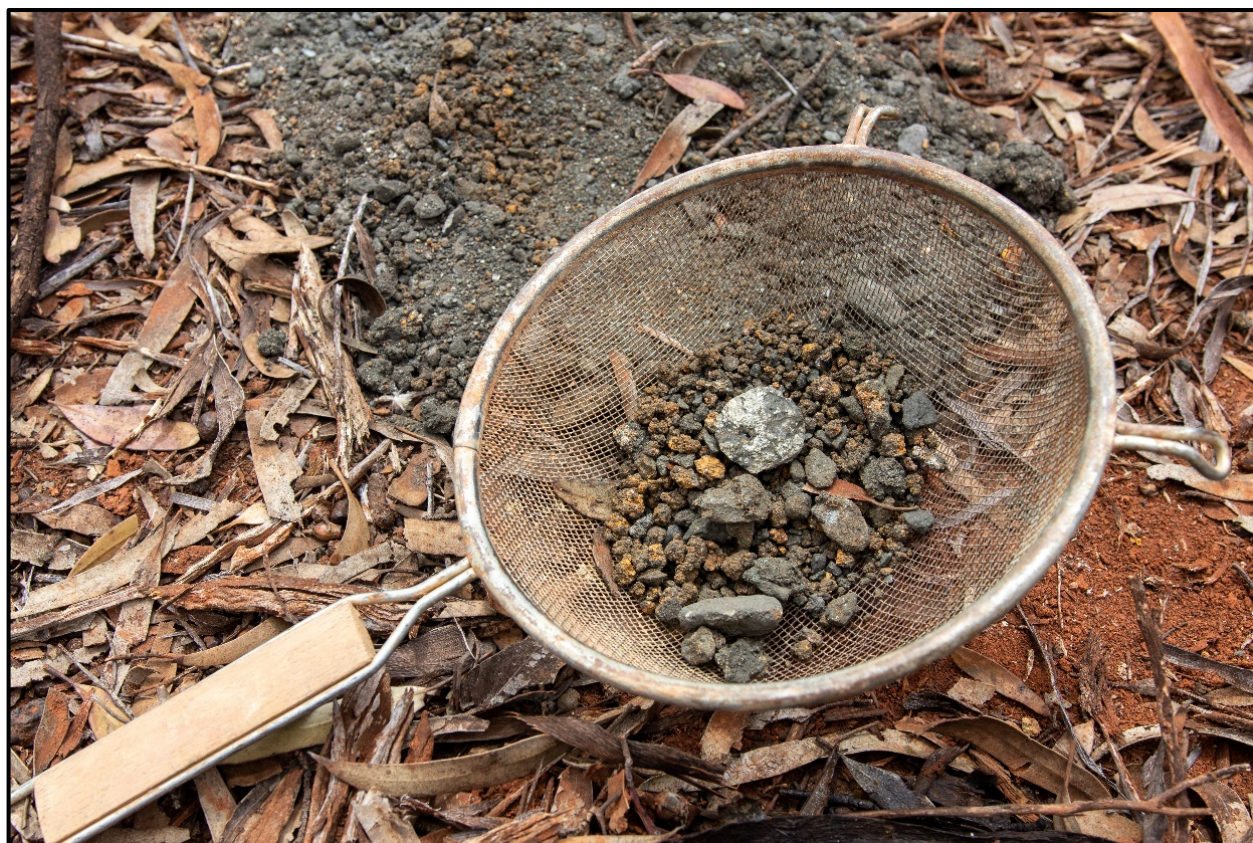
Figure 2 — End of hole aircore sample from NAC105 at 60 metres downhole depth
