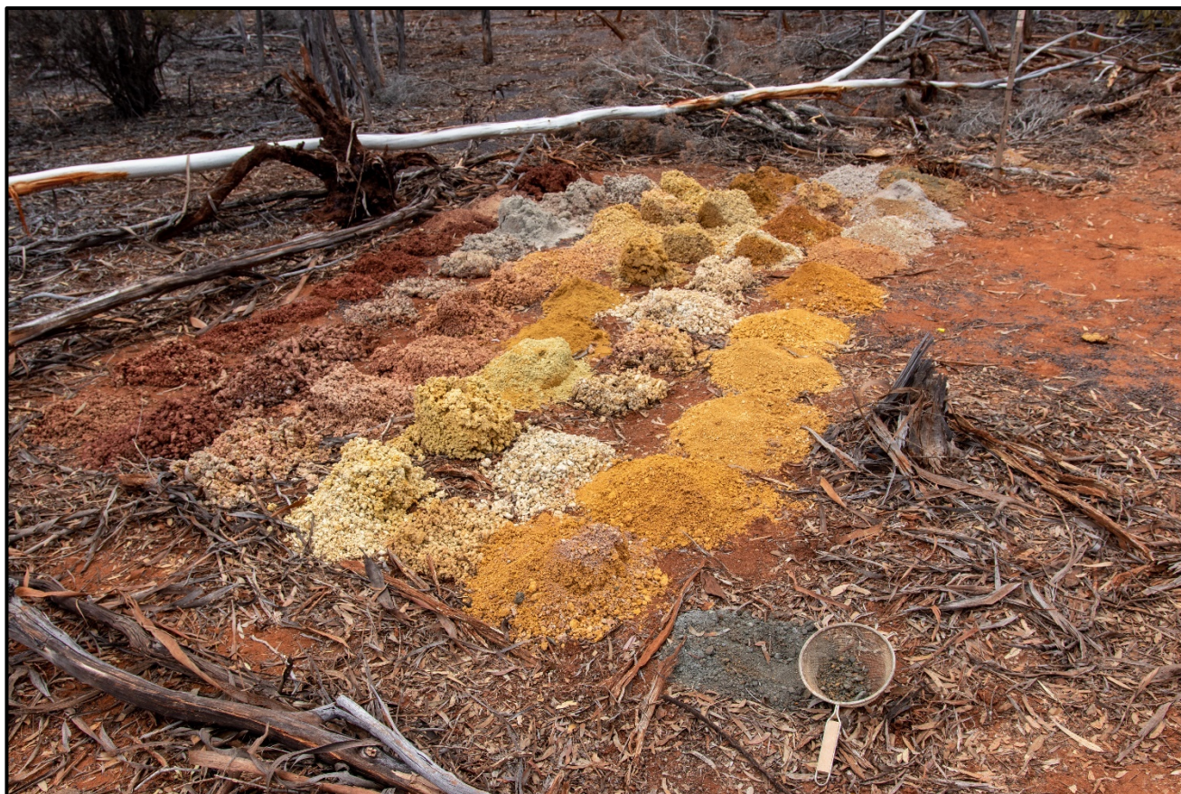
Figure 3 —Aircore drill samples from NAC105 with 1 metre of sulphide mineralisation at the end of hole (right foreground with sieve)
