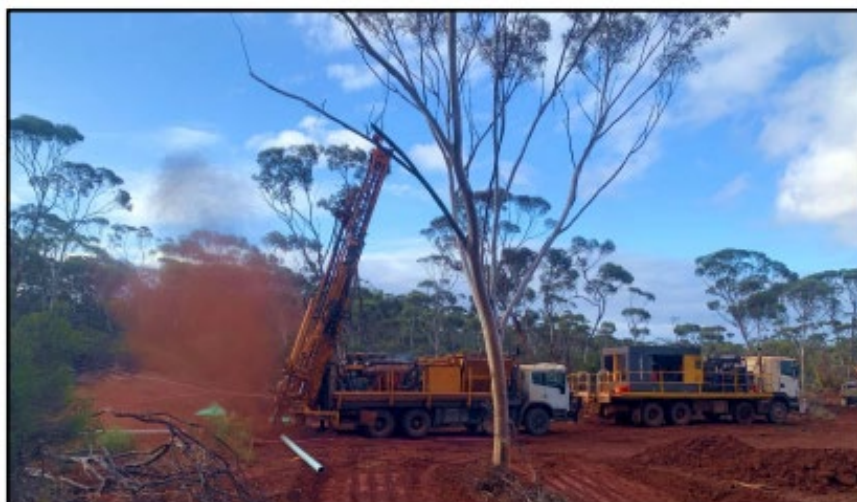
Figure 1: RC Drilling Underway at Galileo's Callisto Discovery near Norseman
