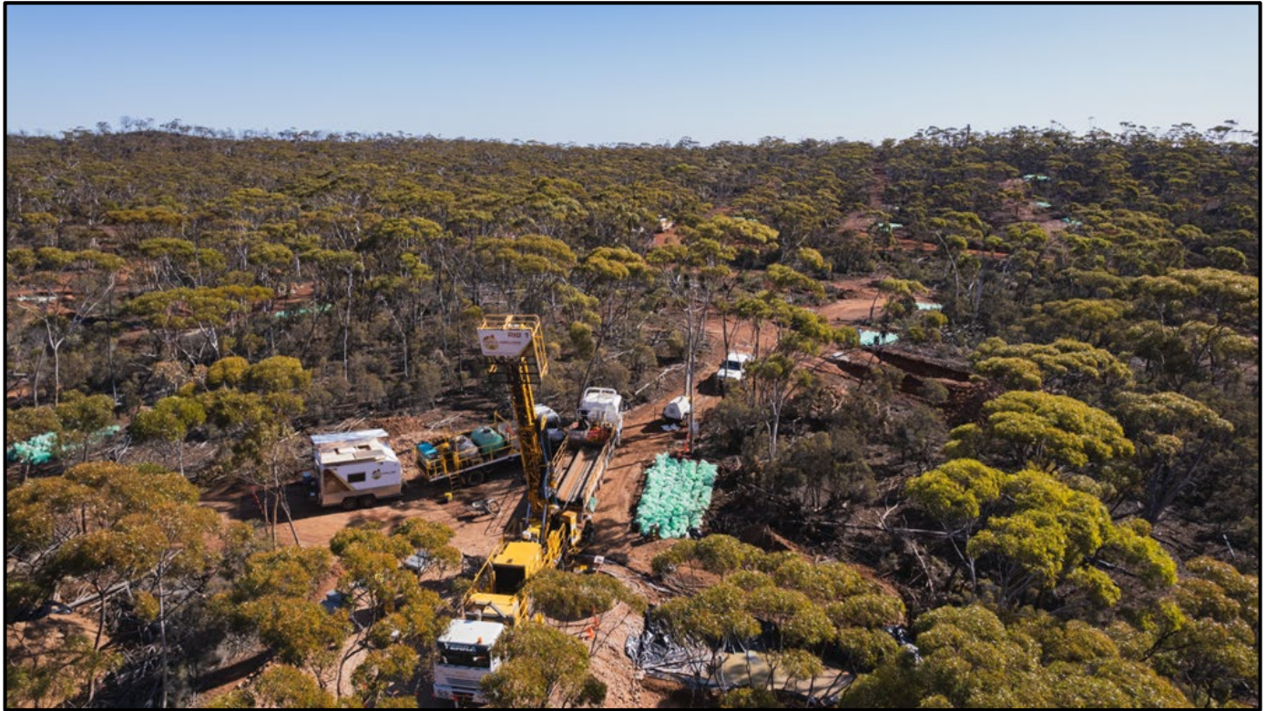
Figure 1 – Diamond core drilling on site at Callisto with completed drill sites in the background. Drill pads and track clearing are designed to minimise the environmental footprint of drilling. All diamond core holes to date have been pre-collared with RC drilling which saves time and money.
