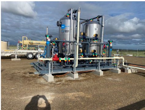
Figure 2: Low pressure gas dehydrator designed to remove moisture as it passes through two contactor desiccant vessels
