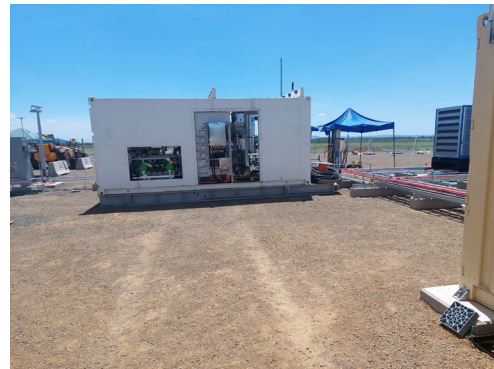
Figure 3: Refurbished Four Stage CNG Compressor capable of 25000 Kpa (3750 psi). CNG in a box
