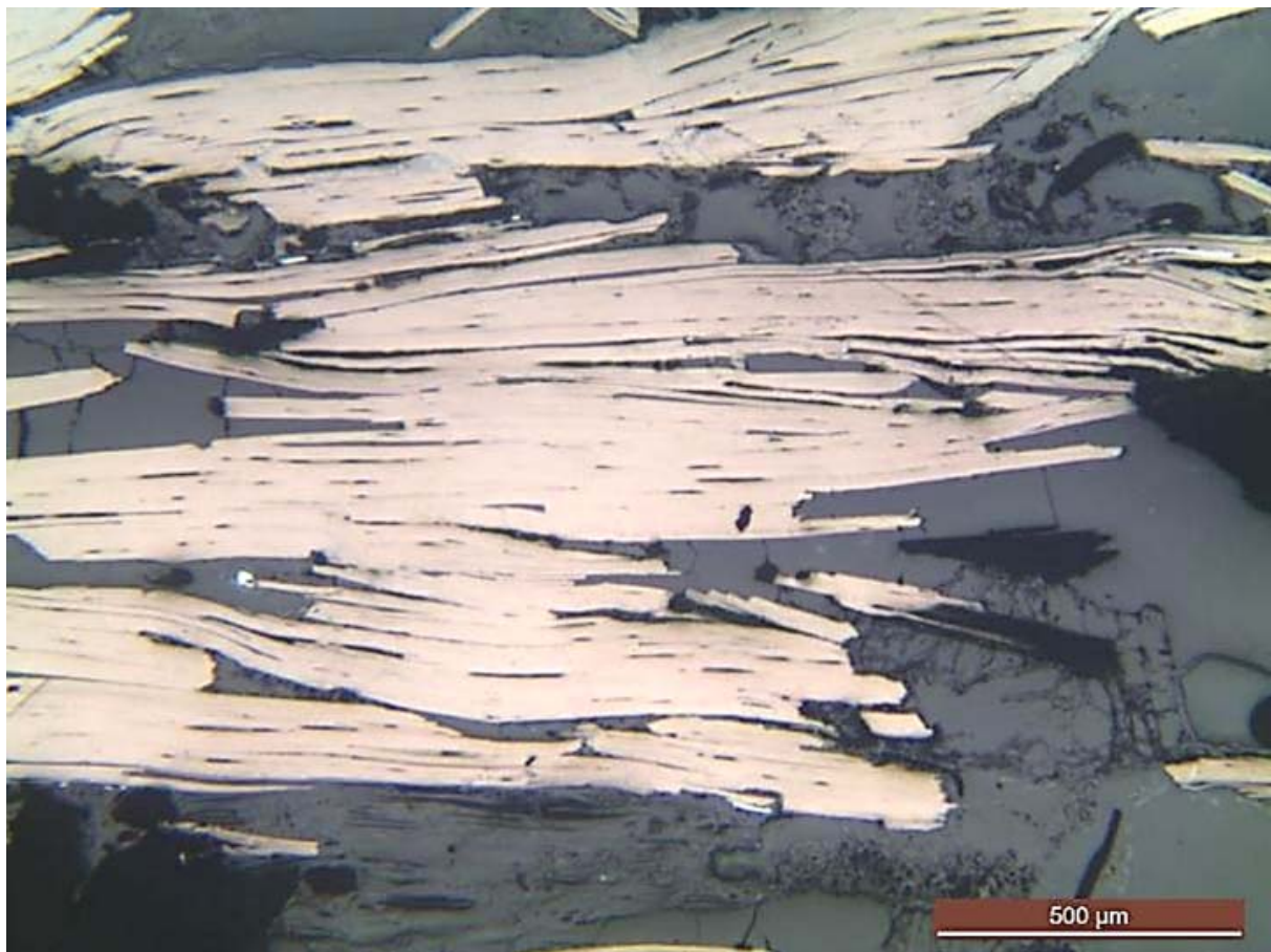
Figure 7. Photomicrograph of Chimutu Prospect Mineralisation (Bright areas are graphite)
