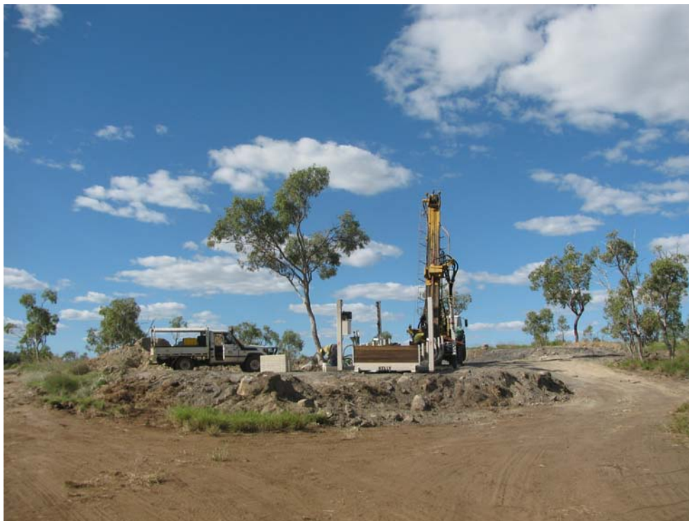
Picture: Diamond drilling at the Milo Prospect.
