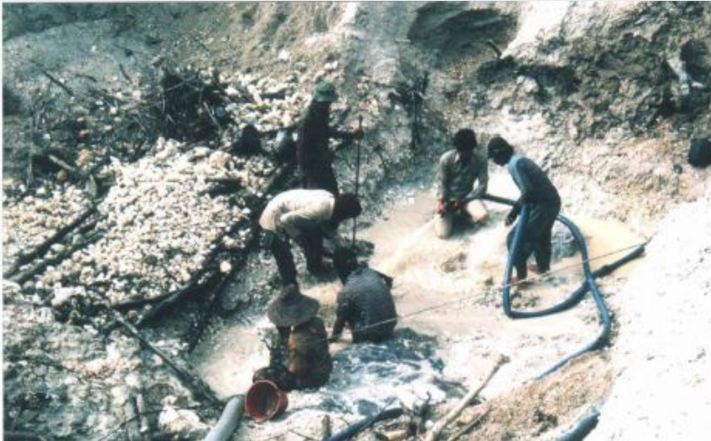
Sluicing at Lubuk Mandi
