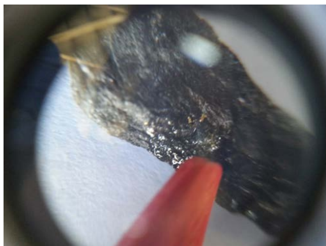
Photographs; Left cluster of native gold particles in quartz vein, right cluster of native gold particles in sheared sediment. Both photographs from LMD010, chinagraph pencil for scale.
