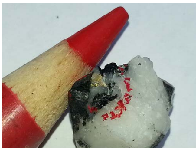
Photographs; Left cluster of native gold particles in quartz vein, right cluster of native gold particles in sheared sediment. Both photographs from LMD010, chinagraph pencil for scale.
