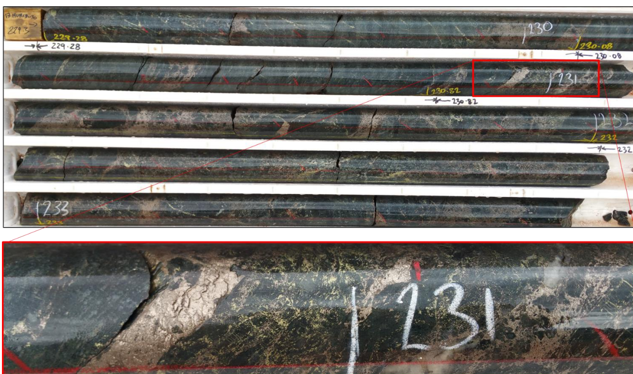
Figure 3. Example of footwall contact lens in hole 17MVRCD030. Enlarged inset shows typical chalcopyrite and pyrrhotite mineralisation proximal to the footwall shear zone
