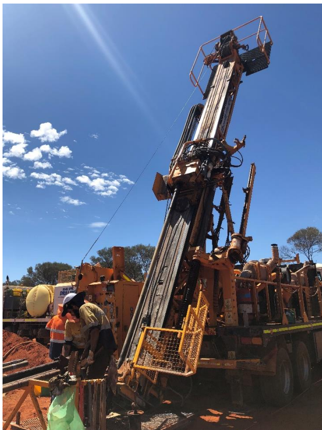
Figure 1. Diamond drill rig on site at Mt Venn (18MVDD001)
