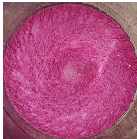
Figure 2. Cobalt Sulphate crystals produced from SX and crystallisation testwork
