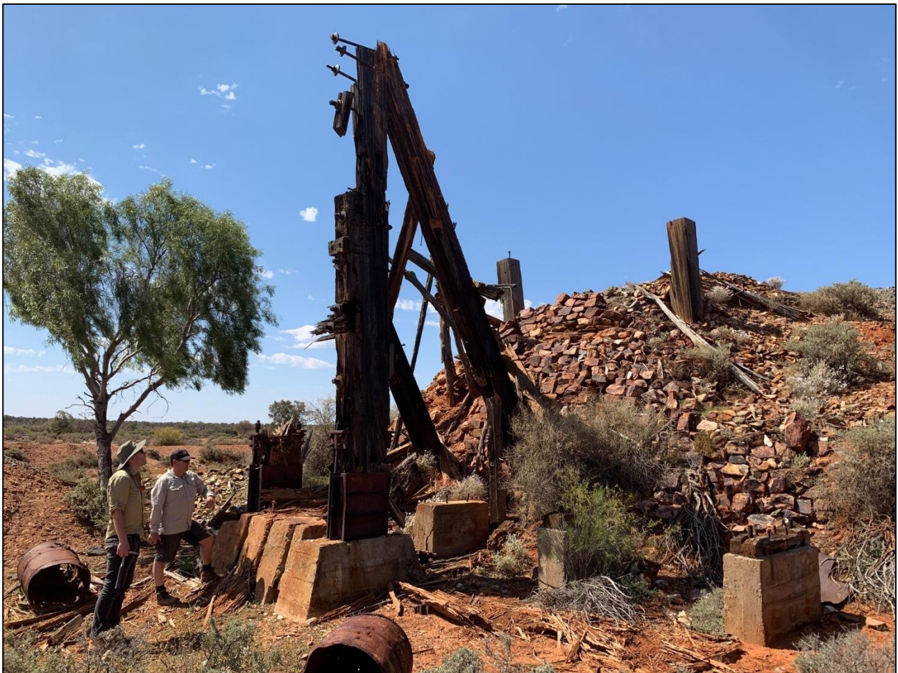
FIGURE 3: REMAINS OF A 3-HEAD STAMP BATTERY AT WHITEHEADS FIND
