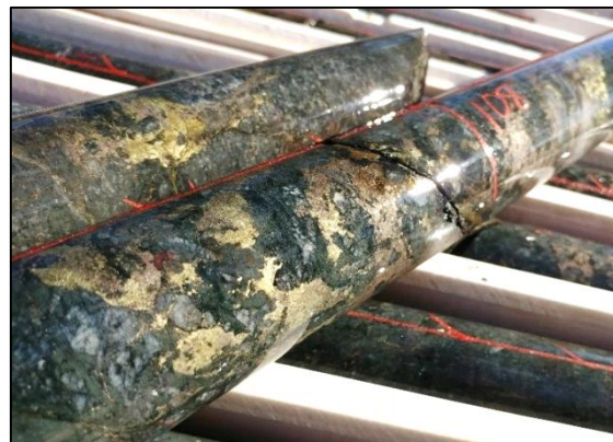
17MVDD003 – Basal contact with interstitial chalcopyrite and pyrrhotite within very coarse-grained gabbro (108m)
