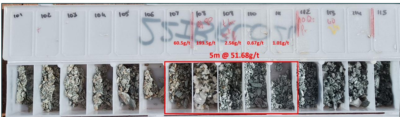
FIGURE 5: RC CHIPS 100 – 115M FROM HOLE 22IBRC024. ASSAY PPM VALUES ARE LABELLED IN RED.
