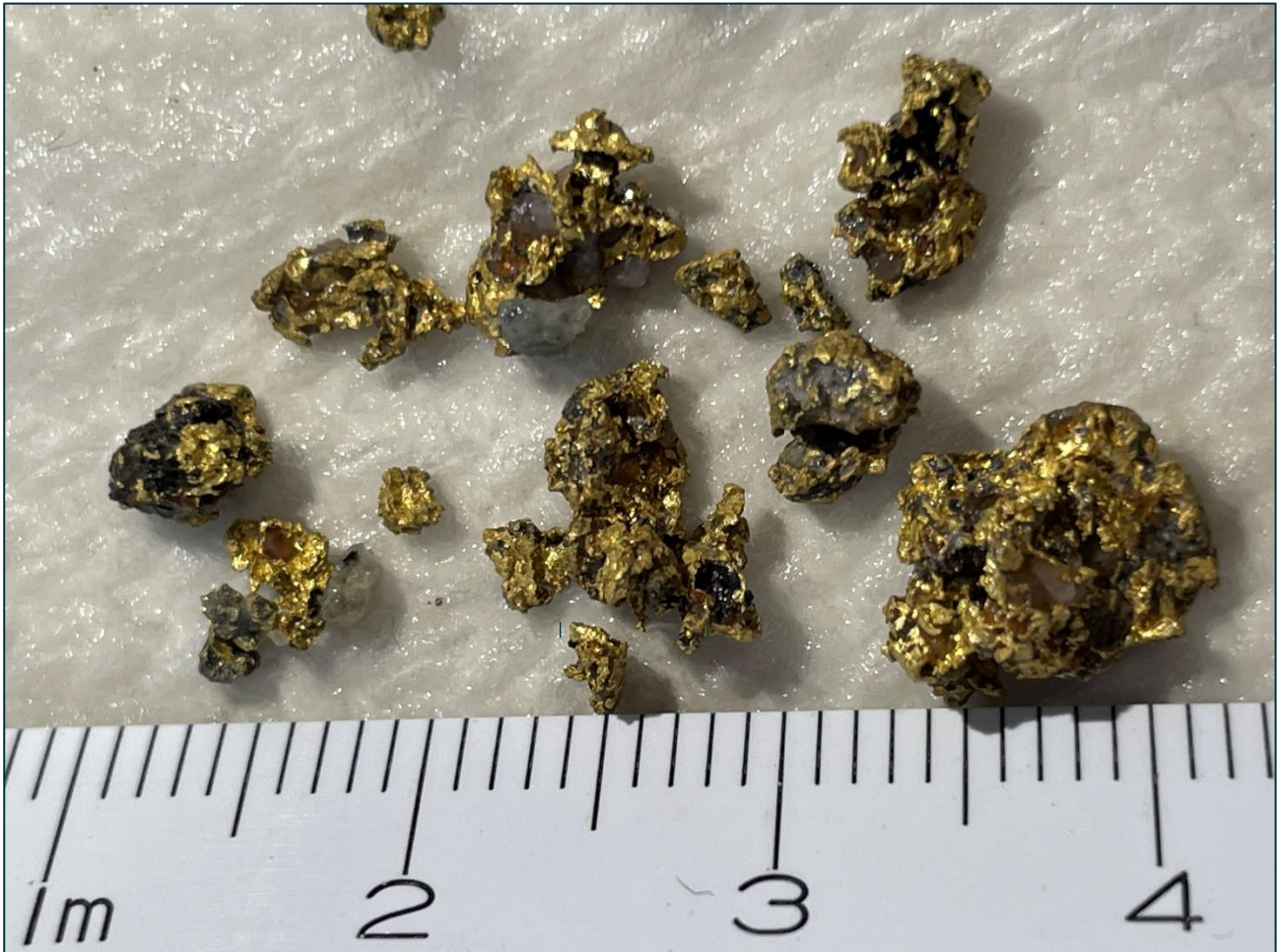
FIGURE 3: COARSE GOLD SIEVED FROM 23MBRC006A 114 TO 115M. RULER INCREMENTS ARE 1MM.
