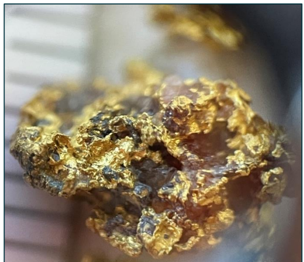
FIGURE 1: COARSE GOLD SIEVED FROM RC CHIPS, 23MBRC006A 114-115M. BACKGROUND SCALE INCREMENTS IN MILLIMETRES. GOLD PARTICLE SIZES VARY FROM 10MM TO SUB-1MM.
