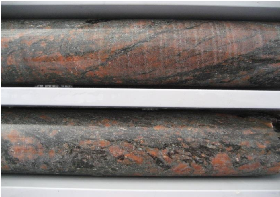
Hematite-dusted K-feldspar and brecciated meta-sediment at 450 metres in hole ALG001
