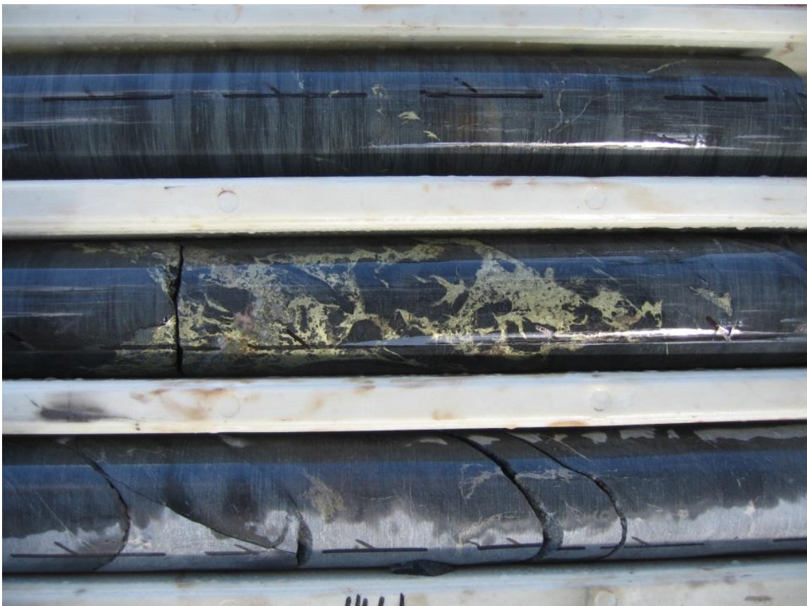
Chalcopyrite and pyrrhotite in core from GCB158 at the Burra Copper Mine
