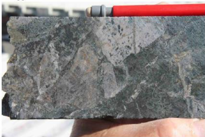
Magmatic hydrothermal breccia with K-feldspar altered clasts and magnetite-chlorite altered matrix. GCHR319. 442.4m. 0.45% copper and 0.24g/t Au.
