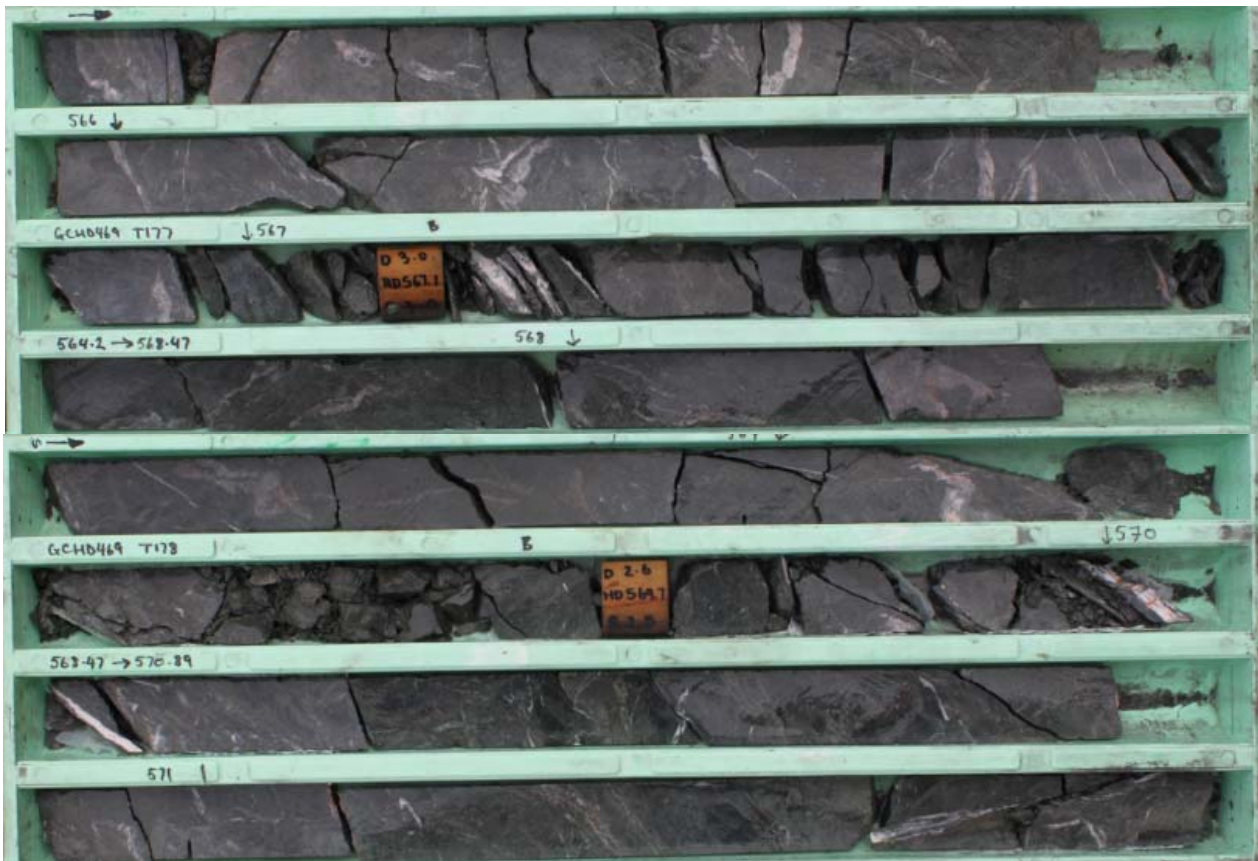
GCHD469 cut core: 565m – 570m, 5 metres at 0.53% copper 0.30g/t gold, hosted by andesitic country rock with quartz-pyrite-anhydrite veining, abundant magnetite-chlorite alteration
