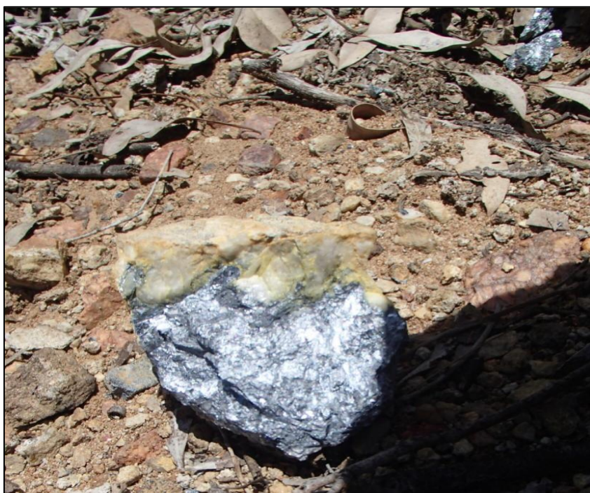
Figure 6: Banshee mine waste dump material observed (unsampled) by Dart Mining in January 2025 showing antimony mineral (70% stibnite*) with encasing vein quartz.*
