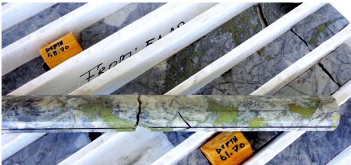
Figure 6– Photograph of strong chalcopyrite mineralisation in drill core from DBDD0001
