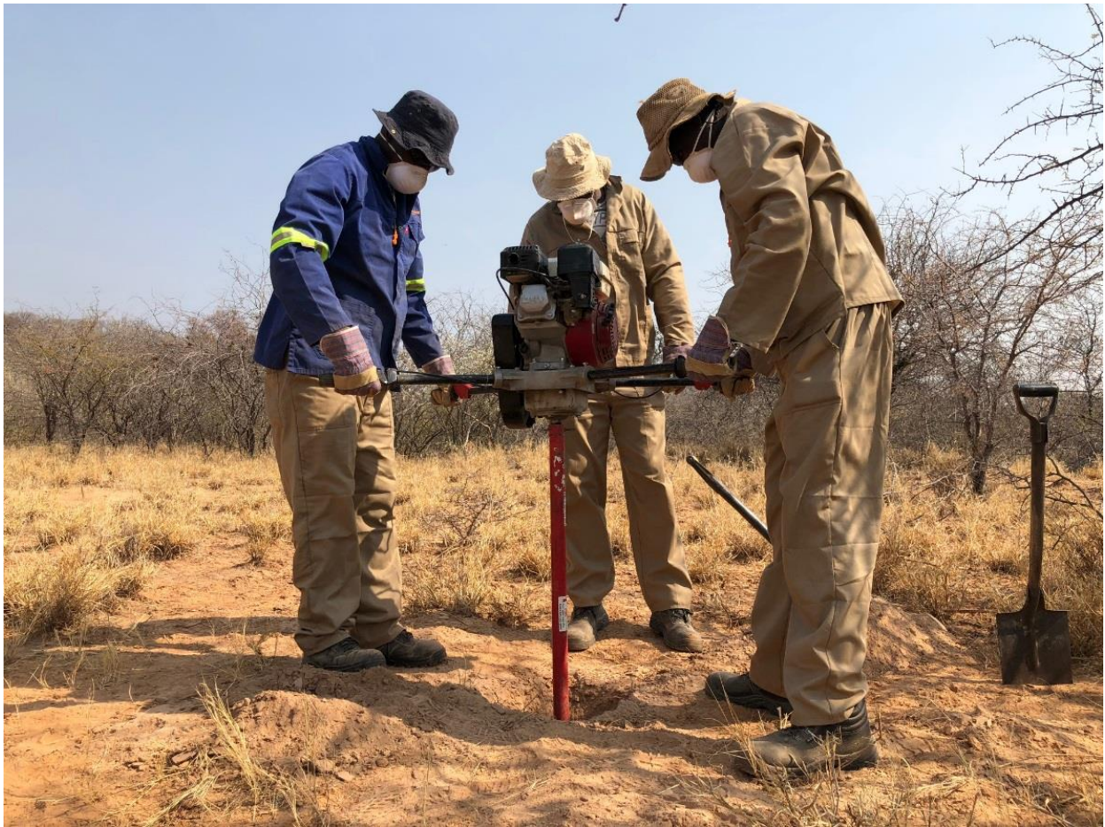
Photograph 1: Auger sampling crew at work on the Abenab tailings
