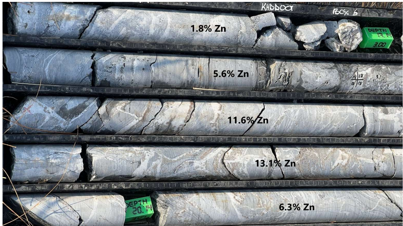
Photo 2: KHDD001, veined and brecciated dolomite with semi-massive sphalerite (zinc sulphide) lenses and veins
