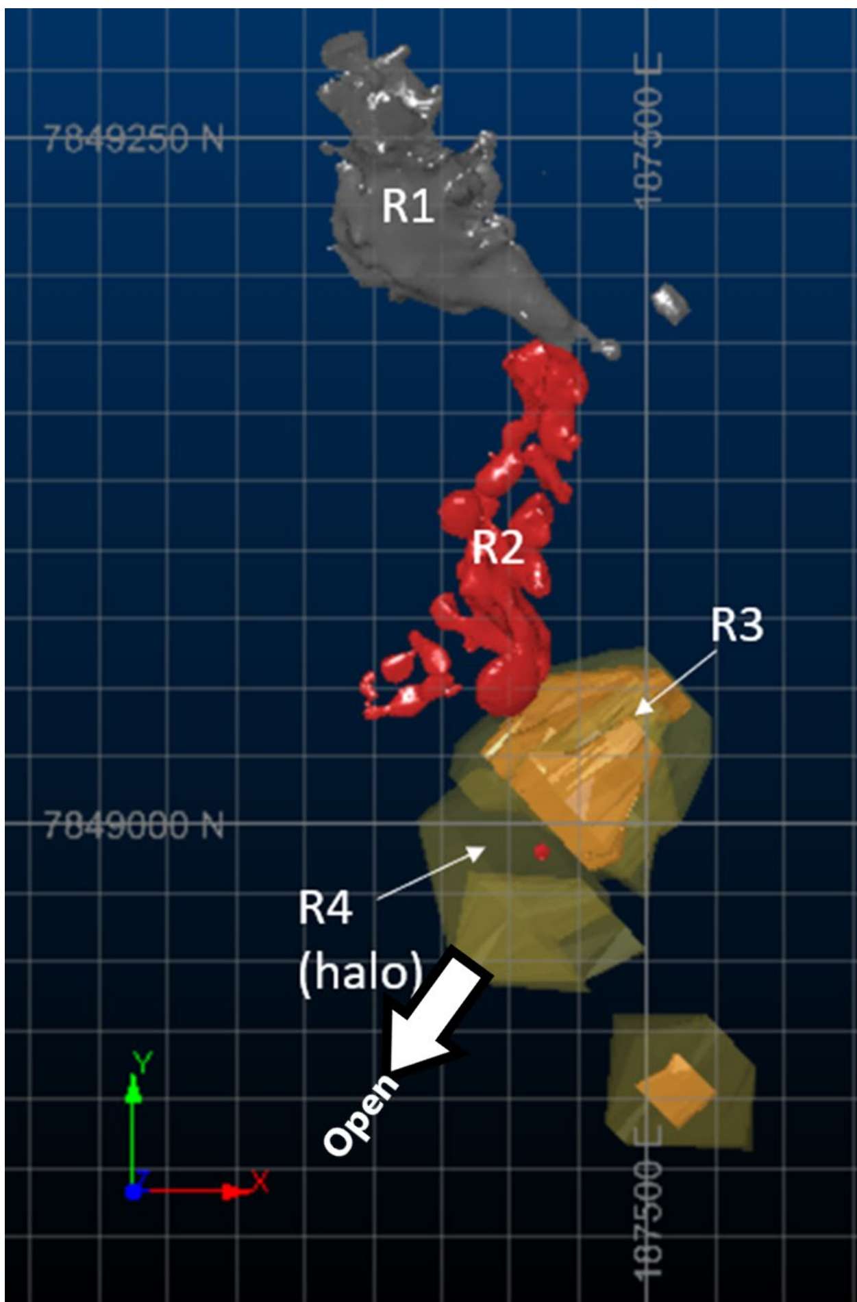
Figure 4: Khusib Springs deposit, plan projection with Mineral Resource model domains
