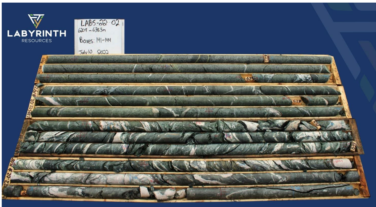
Figure 7 – Visually interpreted Boucher intercept commencing at ~630m
