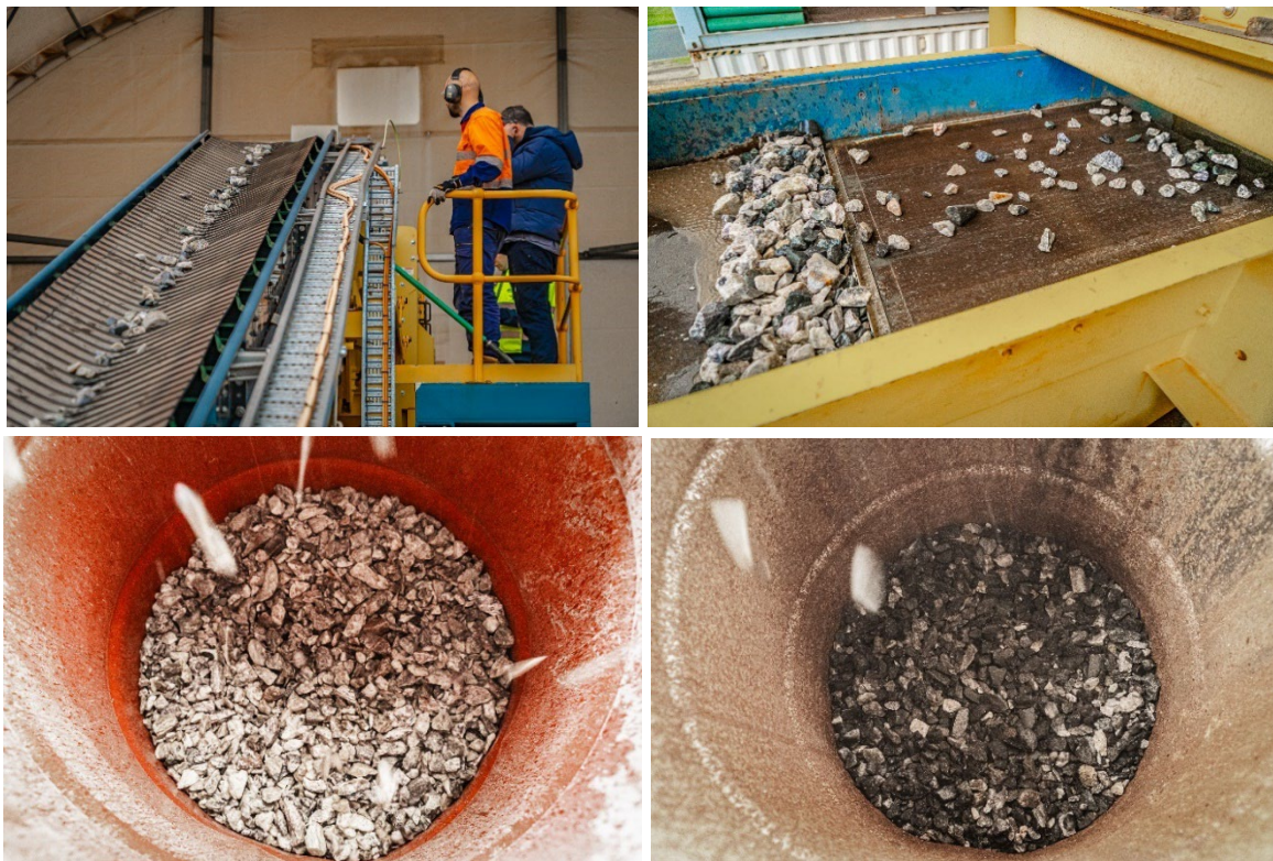
Figure 10. Showing Manna ore being processed through Steinert ore sorting facility.
