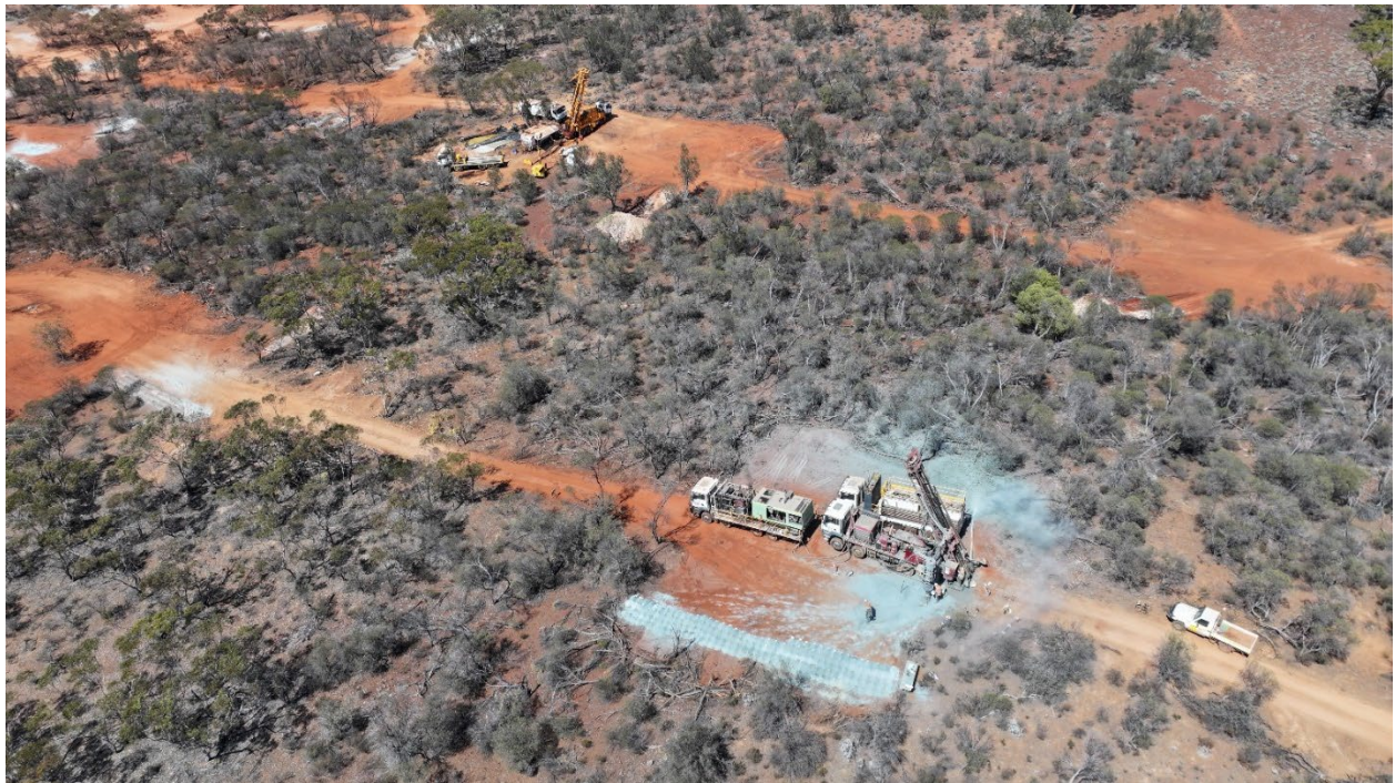
Figure 5. Infill drilling using multiple drill rigs at the Manna Lithium Project.
