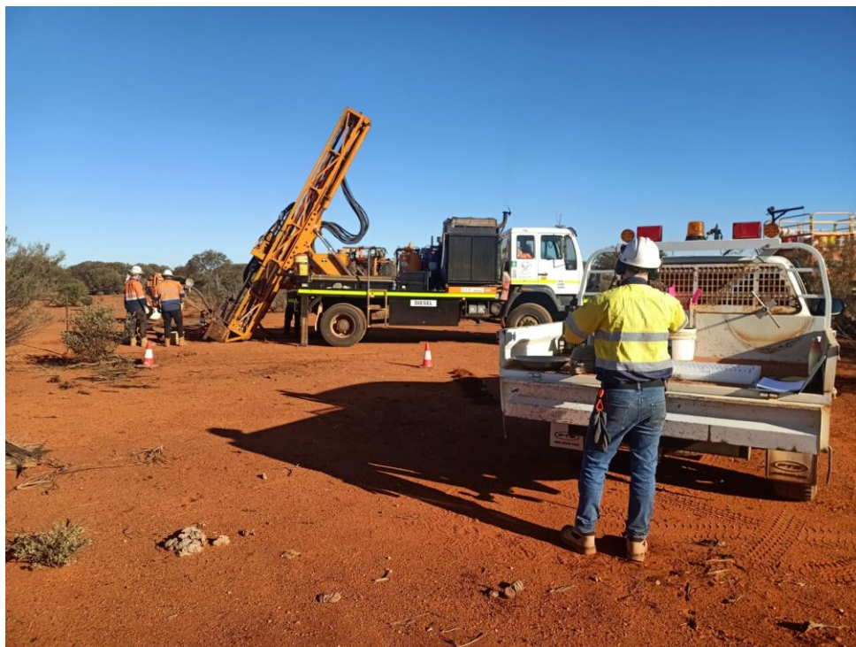
Figure (1): Air-core drill rig on site at the Plymouth North target.
