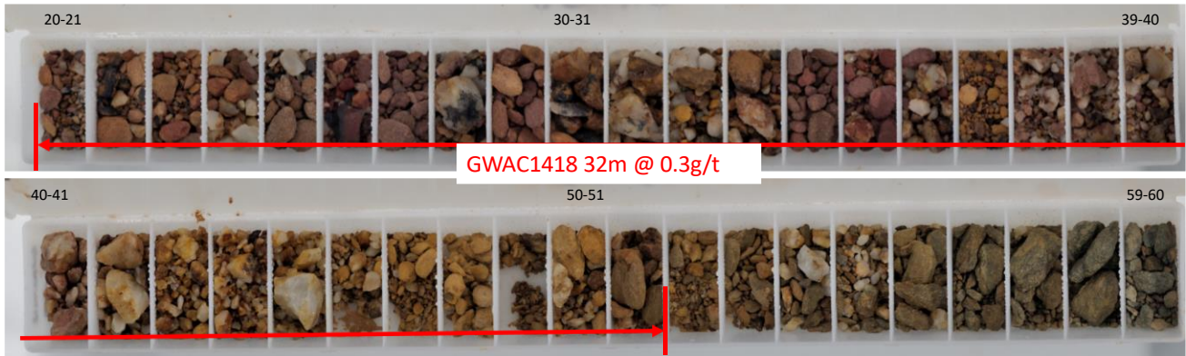
Figure (6): Plymouth north air-core hole GWAC1418 chip trays, illustrating the significant mineralised shear with quartz veining and remnant sulphides.
