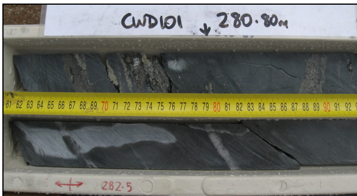
Photo 3 : Pyrite-pyrrhotite-quartz veins, Victoria Lode, CWD101: 280.8m
