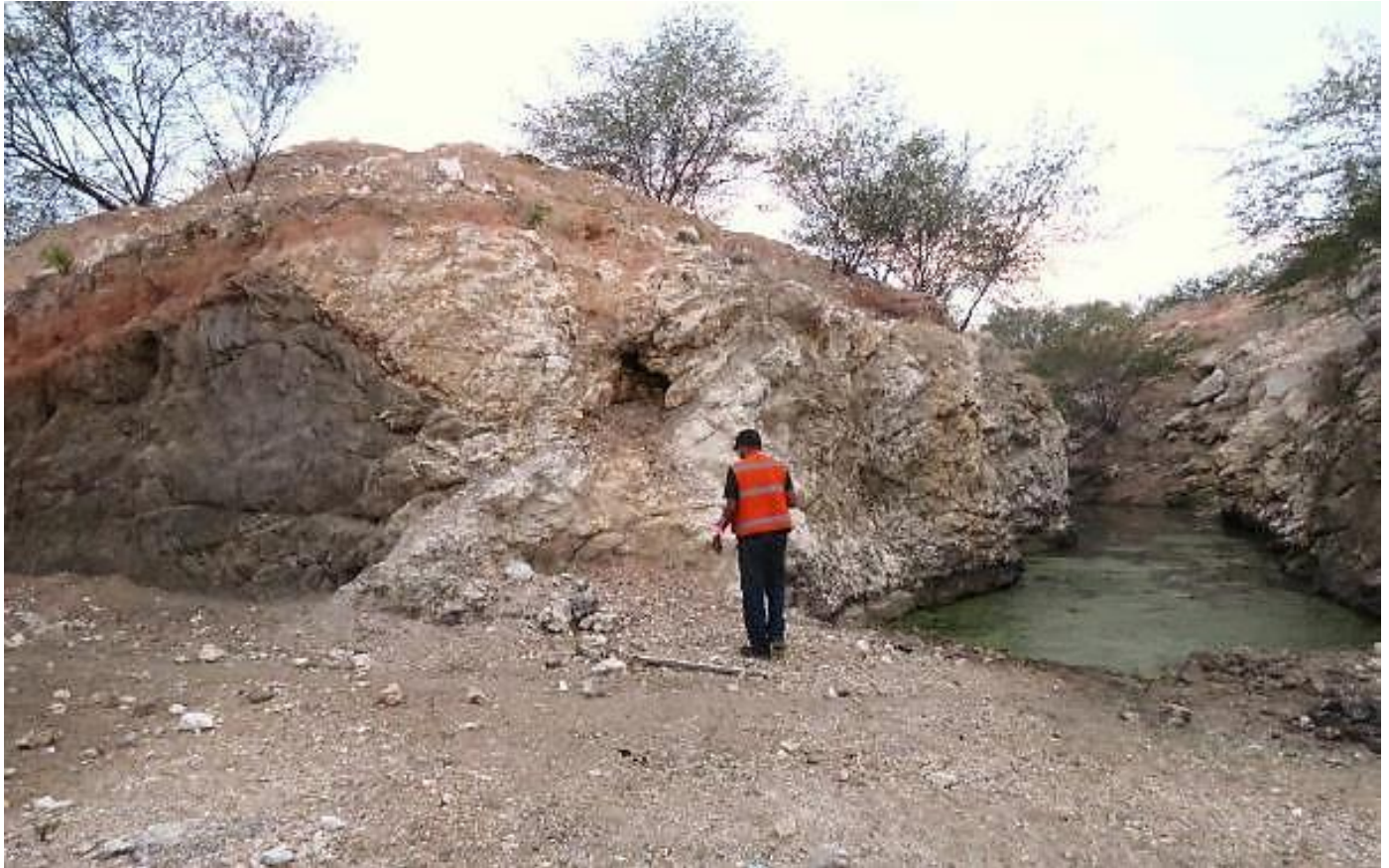
Figure 28. Large pegmatite at an unnamed 32 garimpo in the Seridó Pegmatite Belt. The pegmatite base in the cut leading into the open pit has dips in opposite directions on each side of the road cut on the left of the photo. Trenching on this pegmatite, like many others seen, would not give reliable information on overall dips of the pegmatite.
