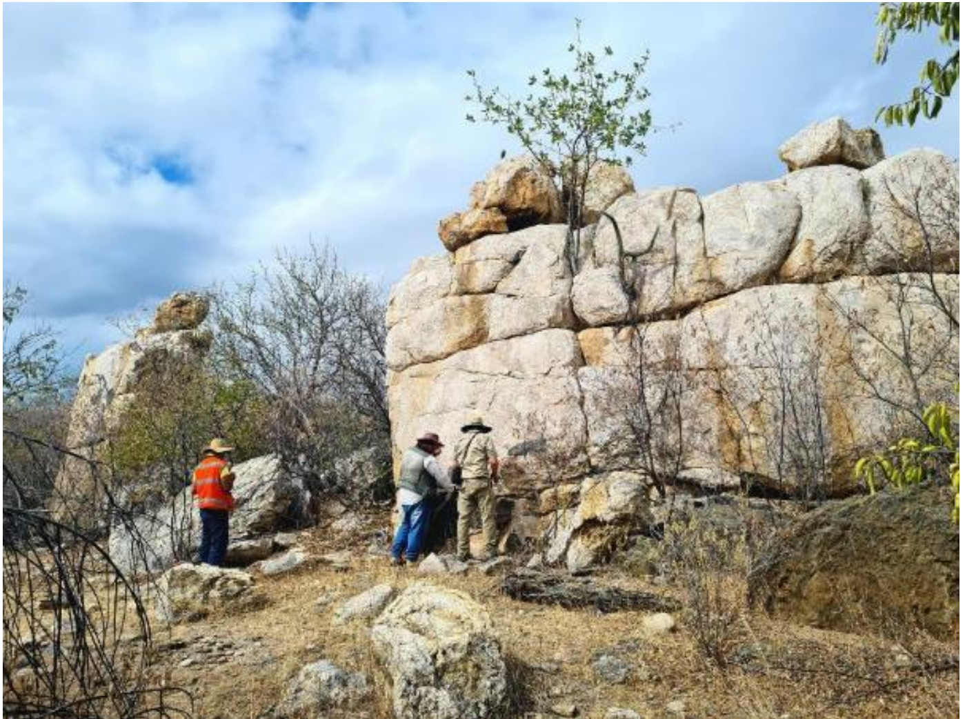
Figure 2. Typical outcrop of an interpreted and confirmed pegmatite at Logradouro. These are all strongly weathered. Additional barely outcropping pegmatites are also present in parts of the tenements.
