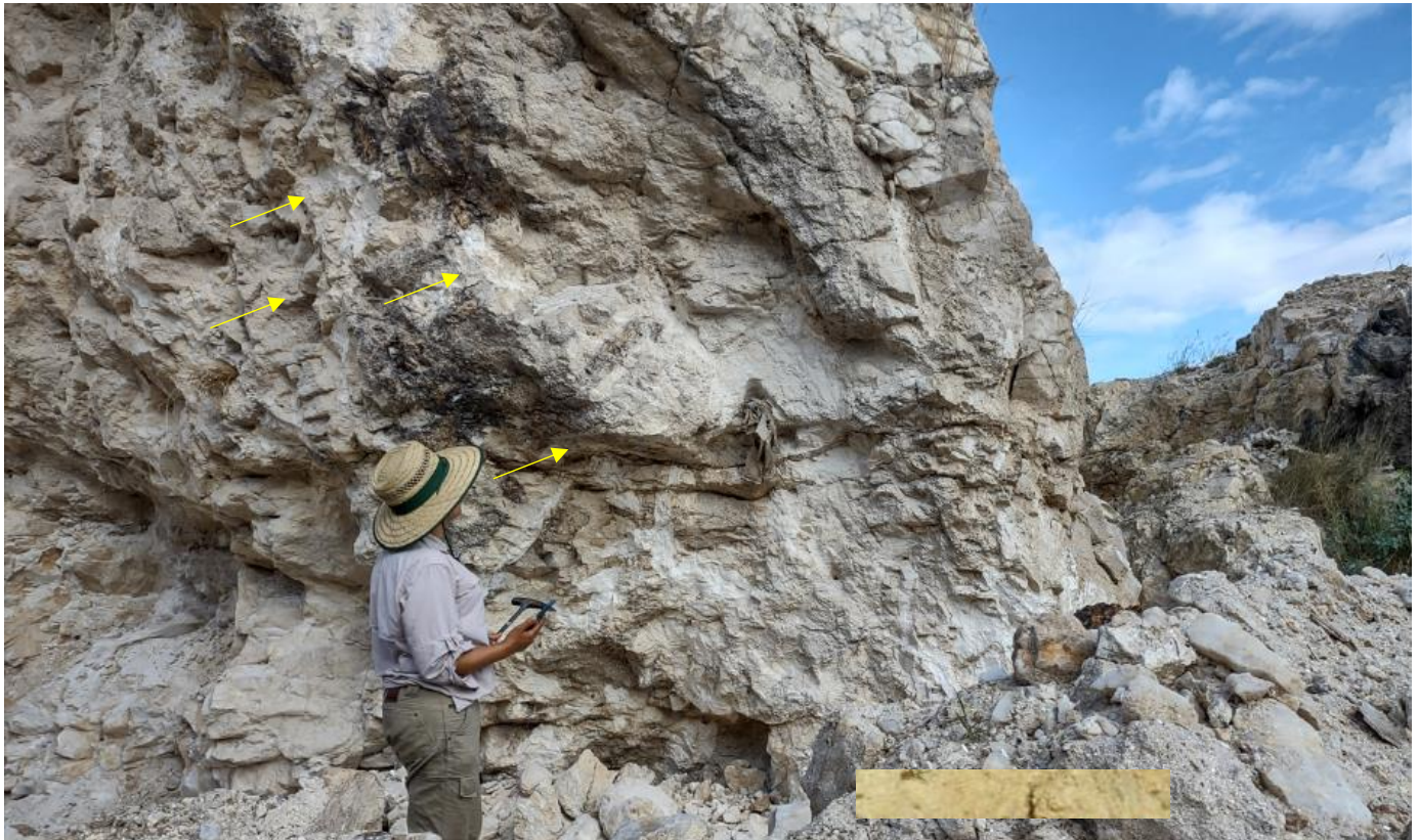
Figure 26. Large tabular bright white pseudomorphs after spodumene at 12-14 metres depth in the Carrapateira mine, (Casa Grande Group) Seridó Pegmatite Belt. Alteration of the spodumene is due to weathering, leaching all lithium and replacing the spodumene by fine grained micas and kaolin. Surface sampling of this pegmatite would not give significant lithium results.
