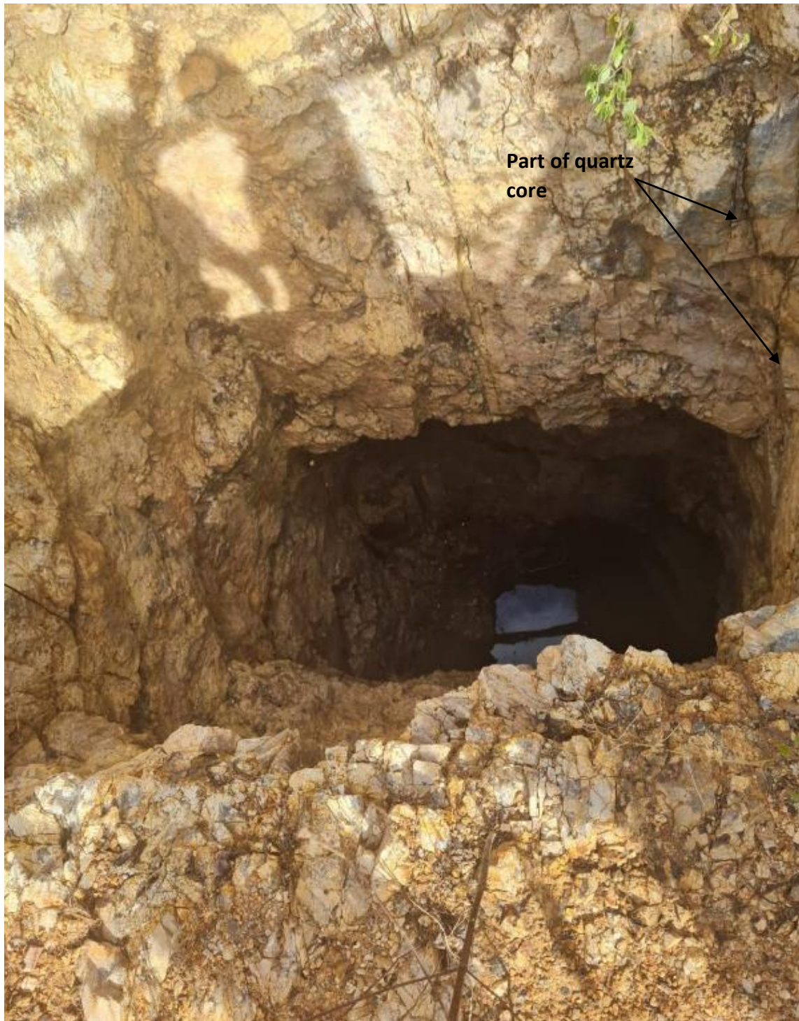
Figure 16. Shaft in the quartz-feldspar dominated pegmatite with the quartz core exposed in the right side of the shaft. Muscovite rich areas were also present at depth. Two rock samples have been taken and dispatched to the laboratory. Results are anticipated in about 2 months.
