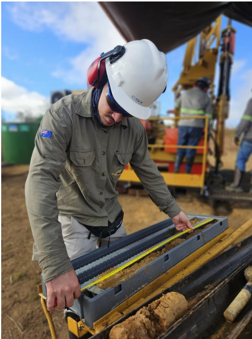
Figure 1. Diamond drilling in prospect IR-1 at Irajuba: measuring recovery on the core.
