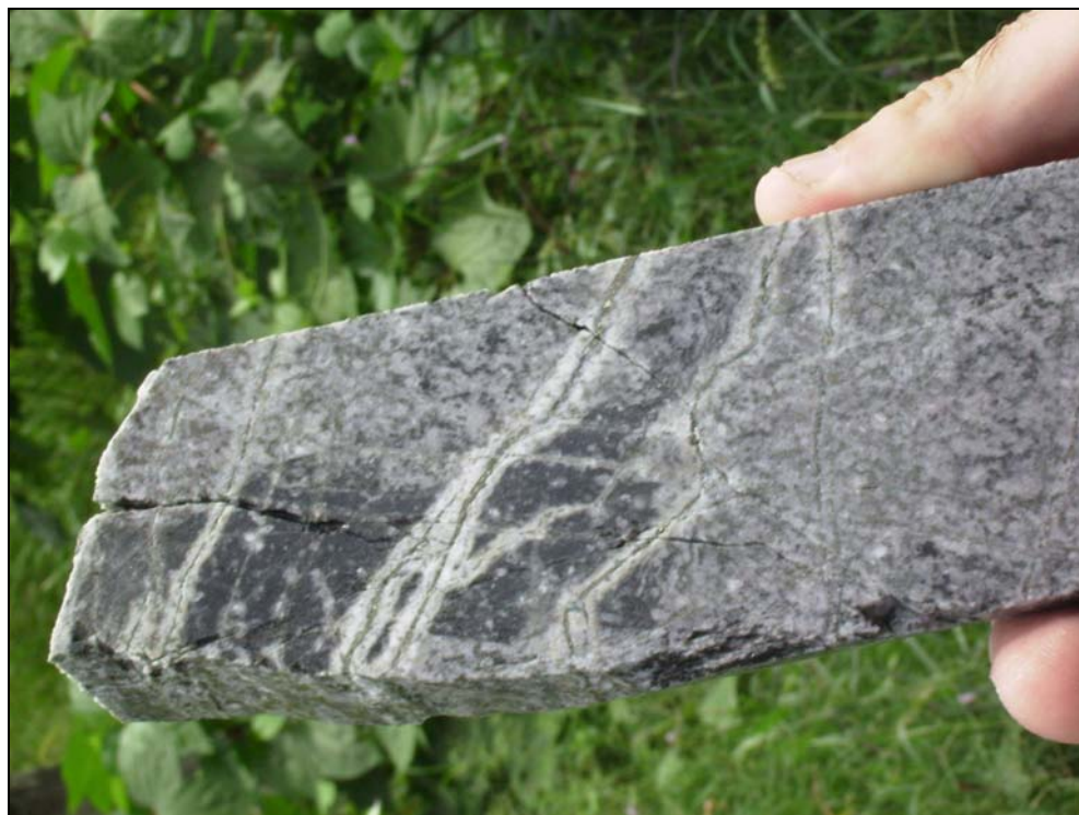
Figure 8. Sawn drill core of DDHNT003 (139m) showing thin sulphide veinlets with selvage alteration typical of porphyry copper deposits.
