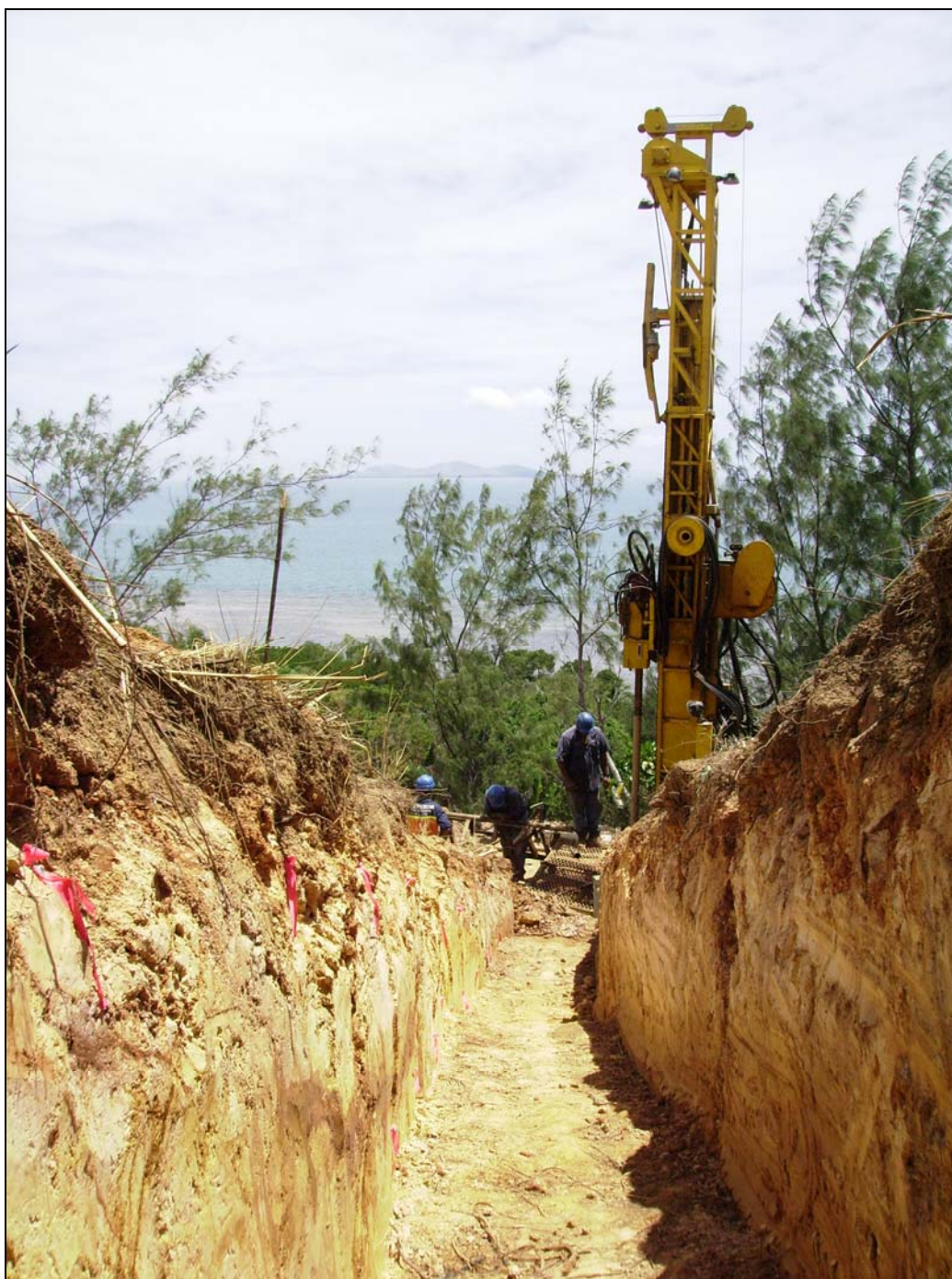
Figure 2. Northern end of trench FT2 at the NE Gossan zone of the Faddy's Gold Deposit. Note that the mineralized gossan is mostly soft, poorly indurated rock and that soil cover is thin. High grade mineralization (1m of 233g/t Au within a zone of 28m of 9.71g/t Au) occurs along this part of trench FT2.
