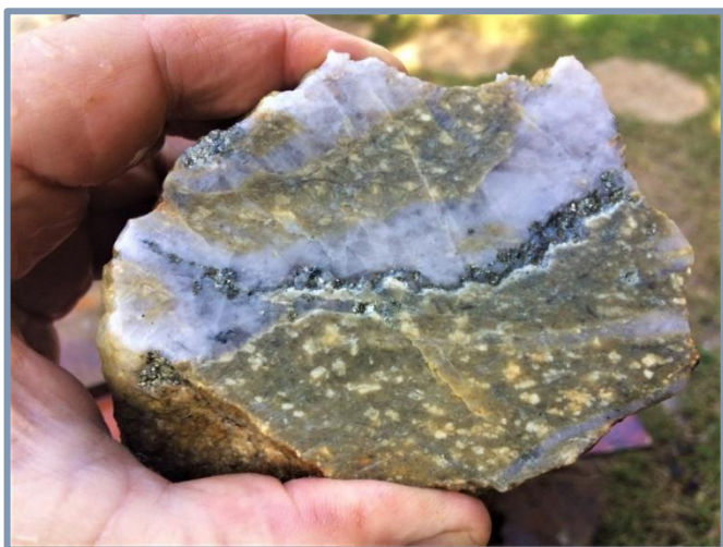
Figure 2: Johnston's Hill stockwork quartz vein with pyrite-galena-gold in intensely silica-sericite altered porphyry
